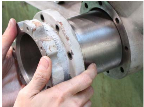
Removing Unloader Cylinder
