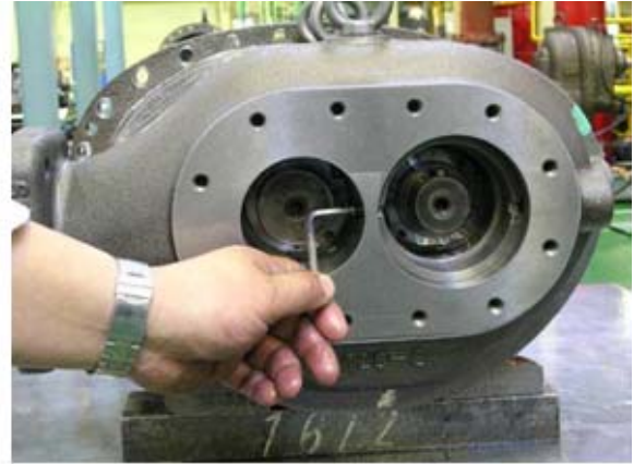
Loosen Hexagon Socket Head Cap Screw for Rotation Stop
