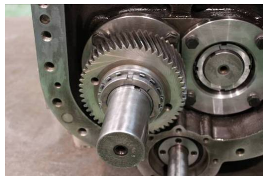
Securing the Speed increaser Driven Gear
