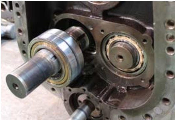
Removing the Thrust Bearing (M rotor)
