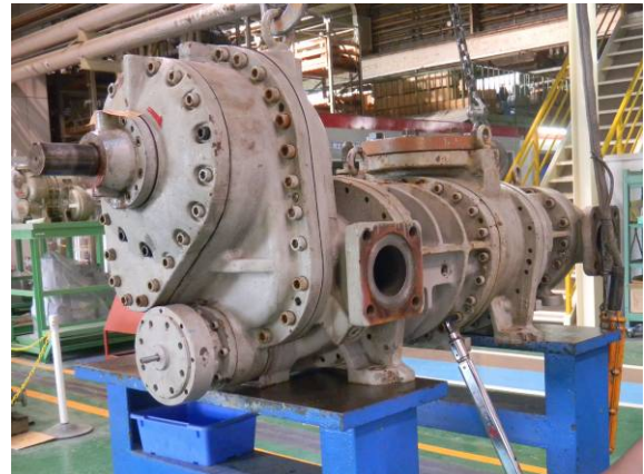
Lower Bolts for Tightening Rotor Casing
