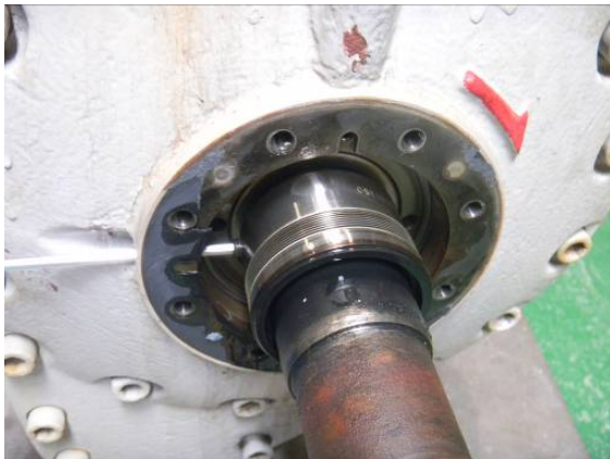
Loosening the Seal Collar Set Screw
