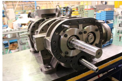
Photo 032 After the Bearing Cover is Removed
