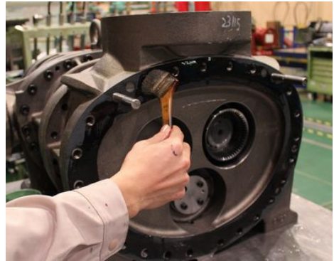
Photo 094 Attaching the Gasket onto the Low-Stage Flange Surface
