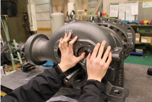
Photo 039 Pulling Out Balance Piston
