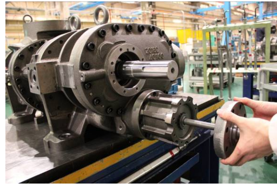
Photo 022 Removing Unloader Cover
