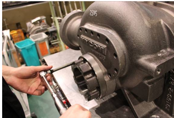
Photo 029 Removing High-stage Unloader Cylinder
