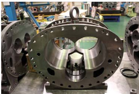
Photo 055 Guide Block Stem Inside Casing
