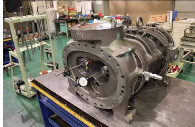
Photo 0868 End Clearance Measurement
