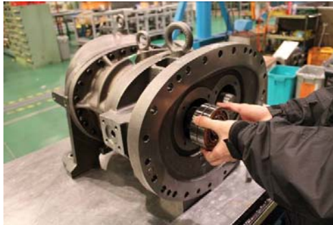
Photo 046 Pulling Out Thrust Bearing
