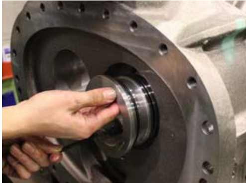
Photo 066 Attaching Side Bearing (Low-stage)
