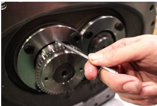
Photo 035 Removing the Driven Hub
