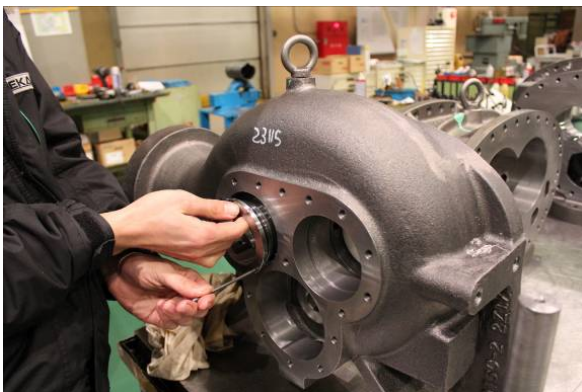
Photo 068 Attaching Side Bearing (High-stage)
