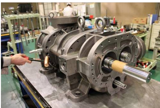
Photo 078 Driving In Alignment Pin for Positioning
