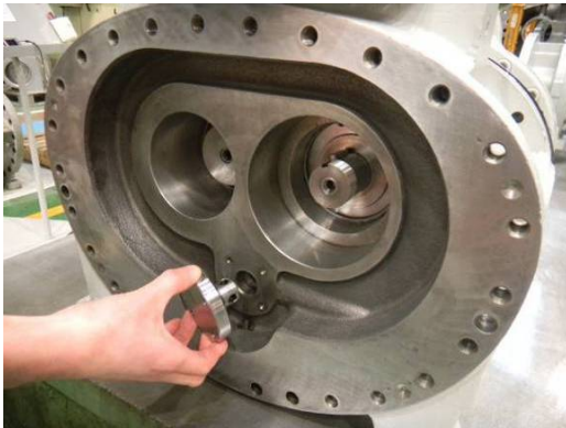
Photo 042 Removal of Oil Injection Pipe Retainer
