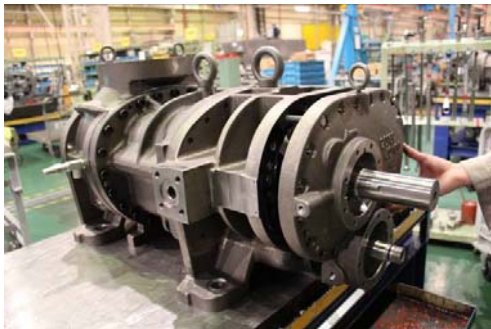
Photo 031 Removing Bearing Cover
