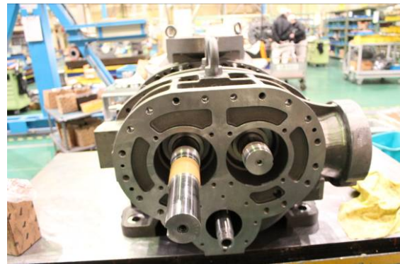
Photo 049 Bearings are Just Removed
