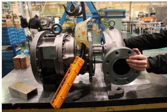
Photo 041 Pulling Out Suction Cover
