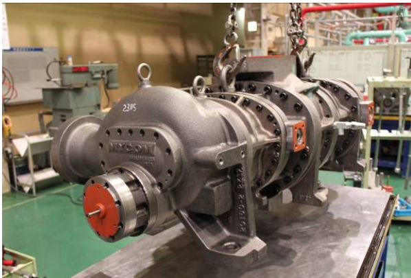
Photo 003 Lifting the Compressor
