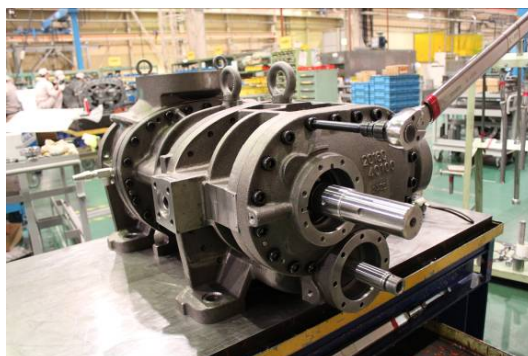
Photo 091 Tightening Bearing Cover
