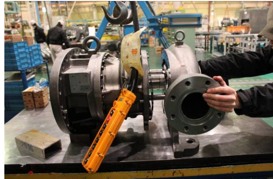
Photo 077 Installing High-stage Suction Cover
