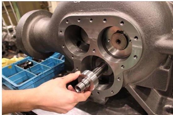
Photo 082 Attaching Load Capacity Adjustment Spacer (Spacer for 20 % Load)
