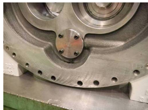
Photo 079 Oil Injection Pipe Retainer
