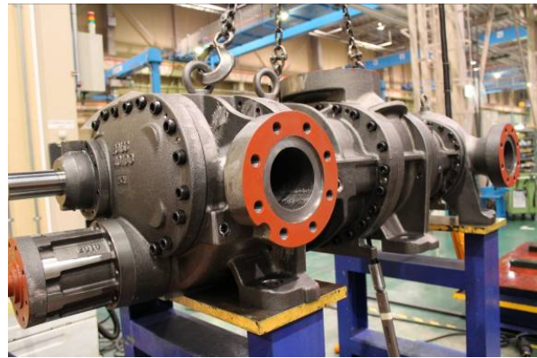
Photo 004 Lower-side Bolts for Fastening Rotor Casing
