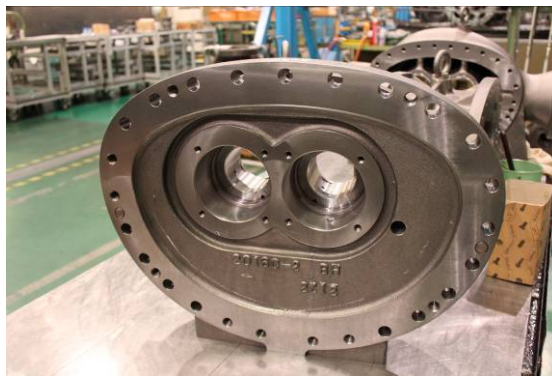
Photo 054 After Removal of Main Bearings
