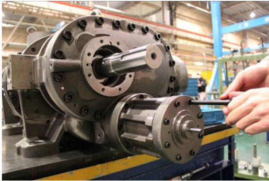
Photo 021 Loosening Bolts of Unloader Cover
