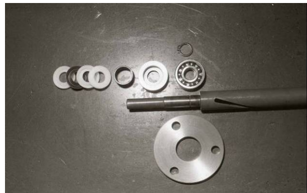
Photo 024 Sealed Portion of Indicator Cam
