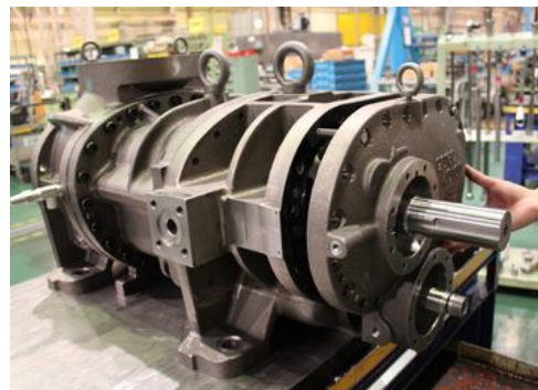
Photo 090 Installing Bearing Cover
