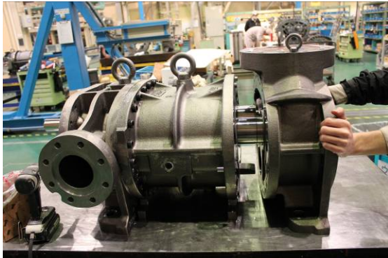
Photo 076 Installing Low-stage Suction Cover
