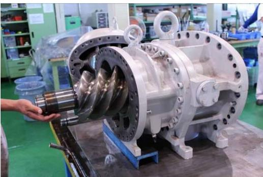
Photo 052 Pulling out M Rotor
