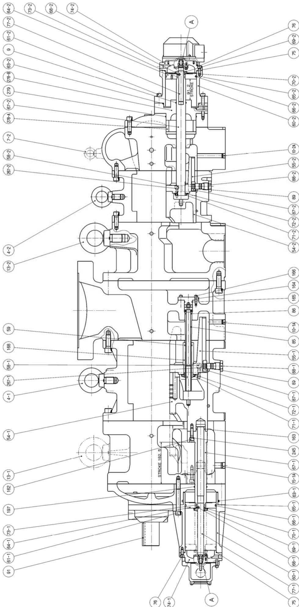
Figure 7-11 2520MSC Assembly Sectional View (Vertical)
