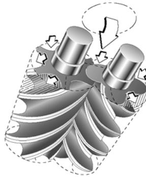
Figure 2-10 Compressor Mechanism
