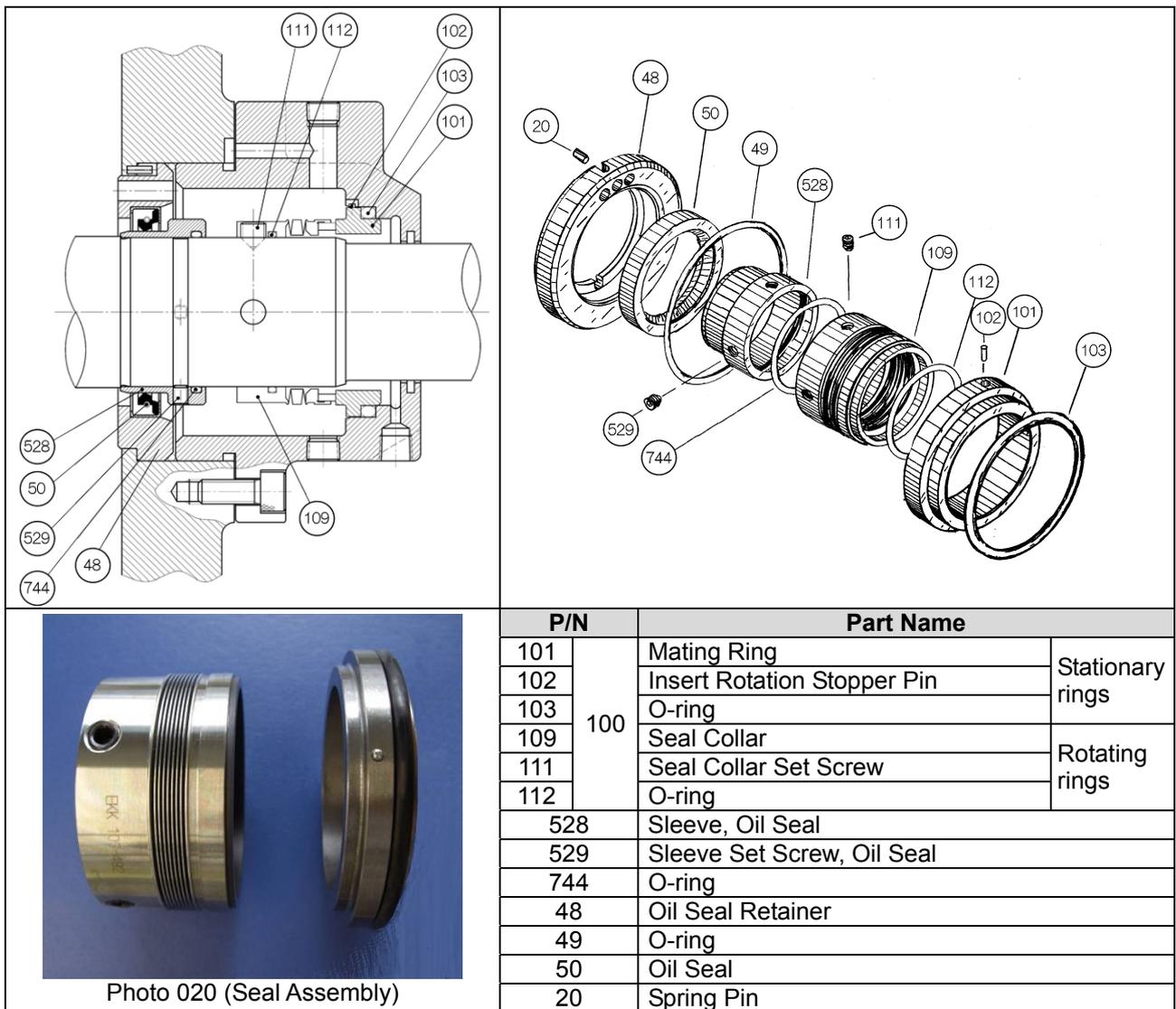
Figure 5-9 Details of BBSE Type Mechanical Seal Assembly and Related Parts
