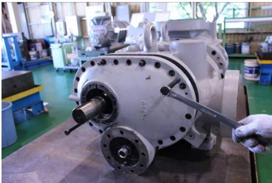
Photo 026 Removing Bearing Cover
