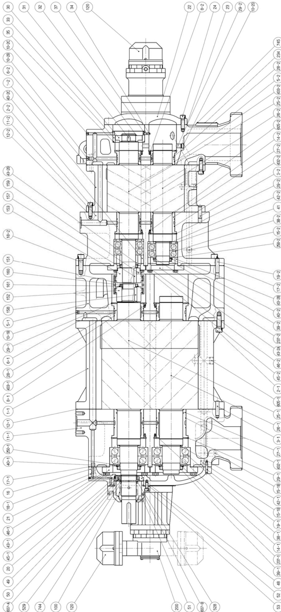
Figure 7-8 2520LSC Assembly Sectional View (Horizontal)
