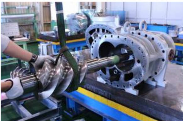
Photo 055 Removing Low-stage M Rotor
