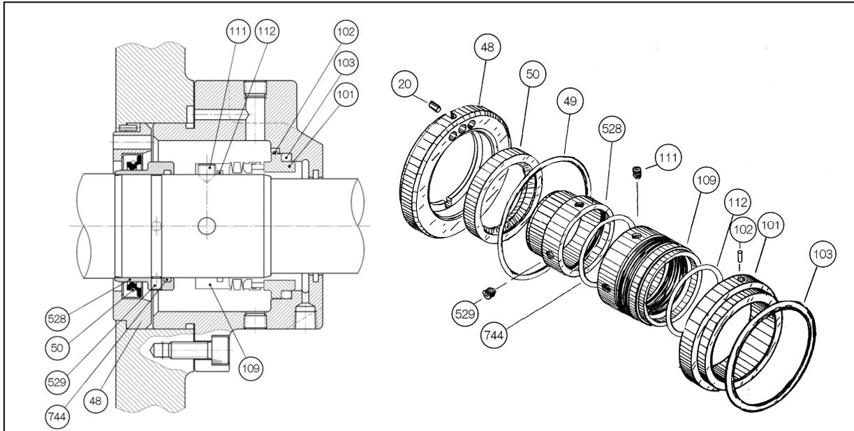
Figure 5-22 BBSE Type Mechanical Seal Assembly
