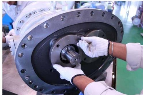
Photo 039 Removing Hexagon Head Bolts
