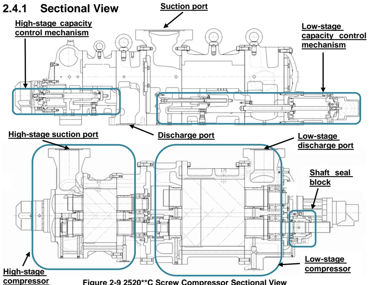
Figure 2-9 2520\*\*C Screw Compressor Sectional View
