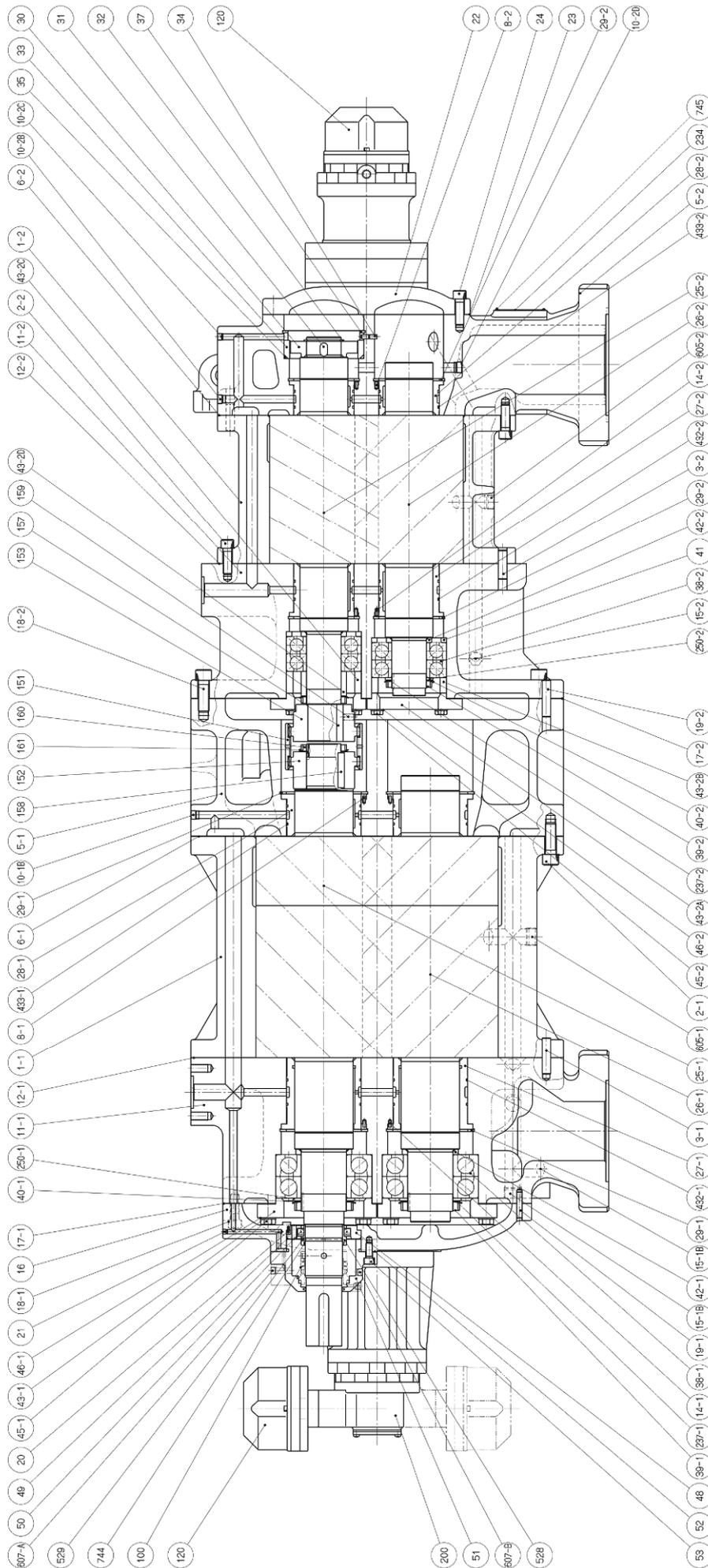
Figure 7-6 2520LMC Assembly Sectional View (Horizontal)
