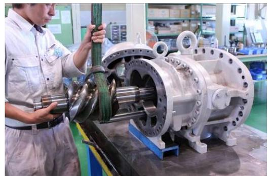
Photo 053 Lifting up M Rotor
