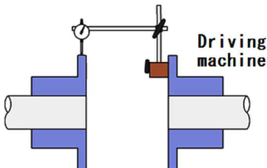
**Figure 3-3 Measurement of Offset**
