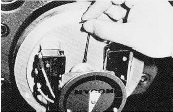
Photo 006 Loosening Micro-switch Cam
