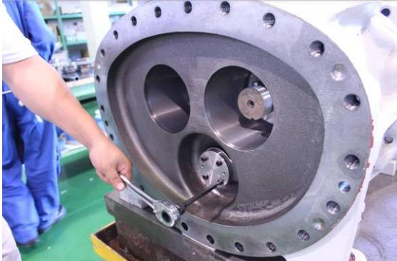
Photo 034 Removing Fastening Bolts
