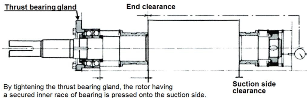
**Figure 5-20 End Clearance Measurement**
