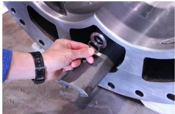
Photo 063 O-ring for Oil Injection Pipe Guide
