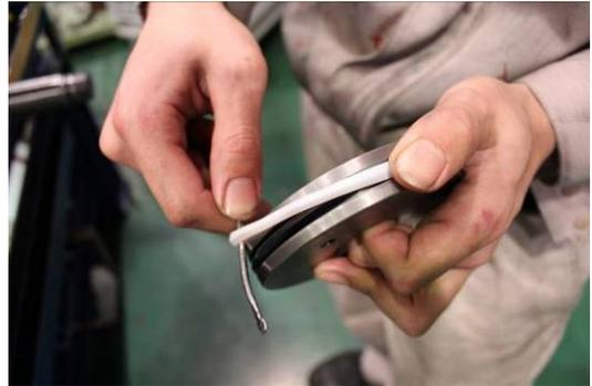
Photo 019 Removing Cap Seal
