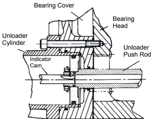
Figure 5-7 Unloader Cylinder Block (Low-stage)
