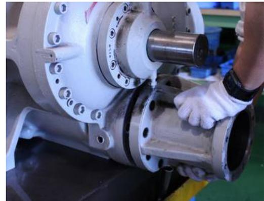
Photo 016 Removing Low-stage Unloader Cylinder
