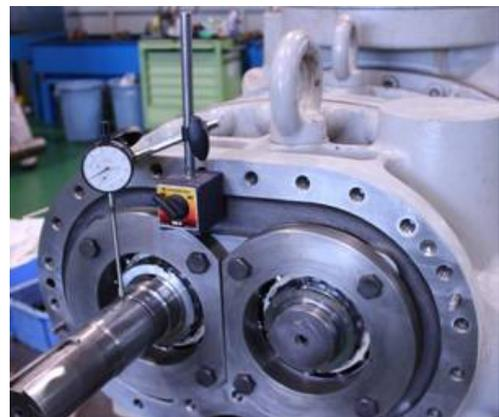
**Photo 098 Measurement of Runout**
