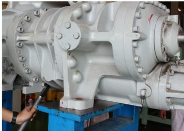
Photo 003 Loosening Lower Flange Fastening Bolts
