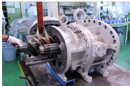
Photo 051 Lifting up F Rotor
