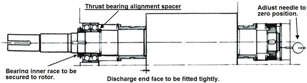
**Figure 5-19 End Clearance Measurement Preparation**
