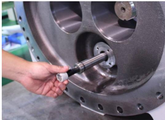
Photo 036 Removing Oil Injection Pipe
