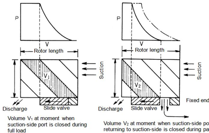
Figure 2-16 Capacity Control Mechanism
