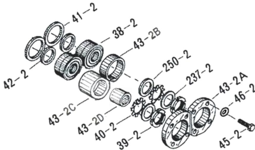
Figure 5-13 High-stage Thrust Bearing Block
