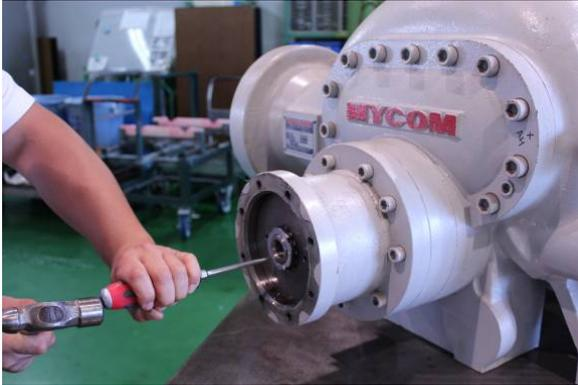
Photo 014 Bending back the Lock Washer Tooth
