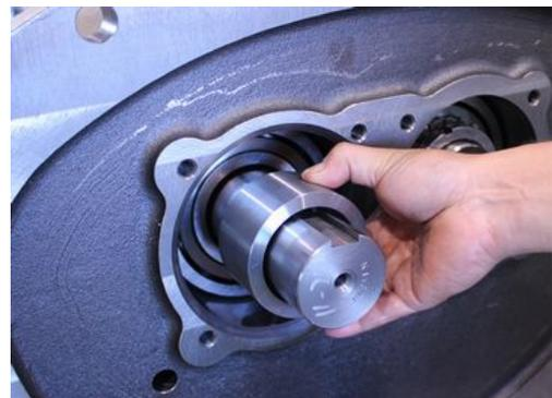
Photo 047 Removing Bearing Gland D
