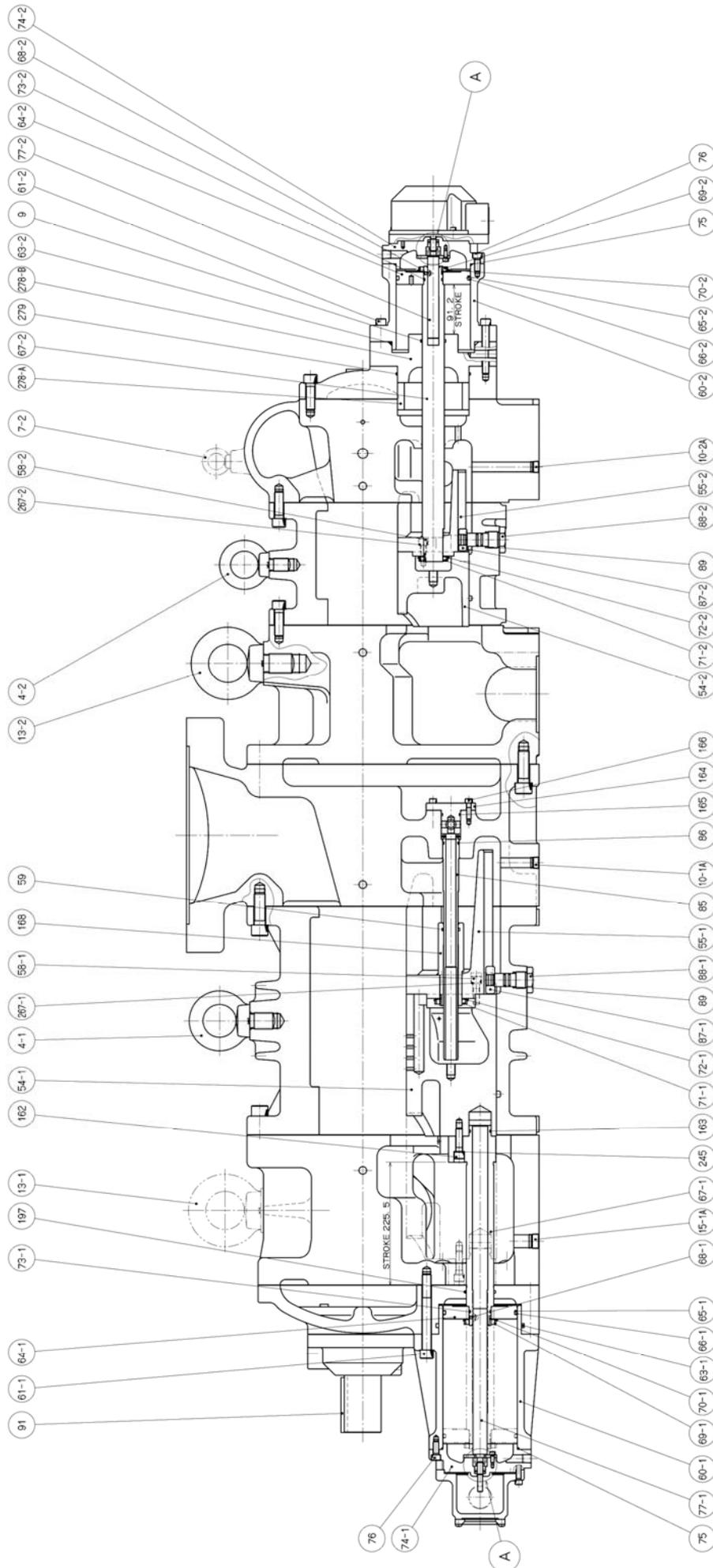
Figure 7-7 2520LSC Assembly Sectional View (Vertical)
