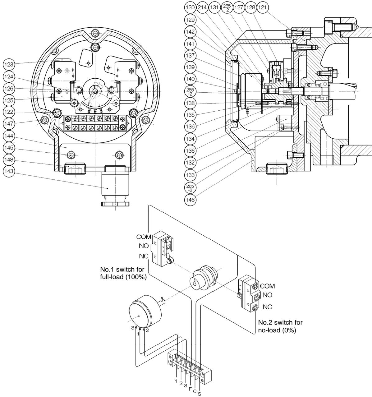
Figure 5-27 Assembly Drawing of Unloader Indicator (Standard type)
