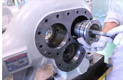
Photo 042 Removing Side Bearing
