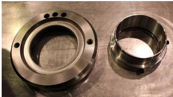
Photo 025 Oil Seal Retainer and Oil Seal Sleeve attached with O-ring
