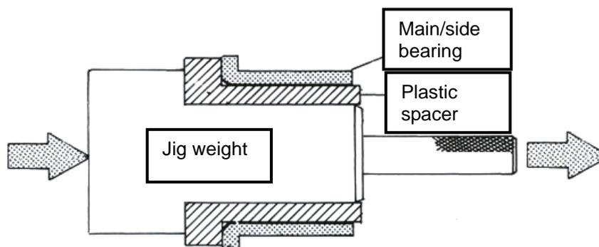
Figure 5-17 Jig (example) for Press fitting Bearing Installation
