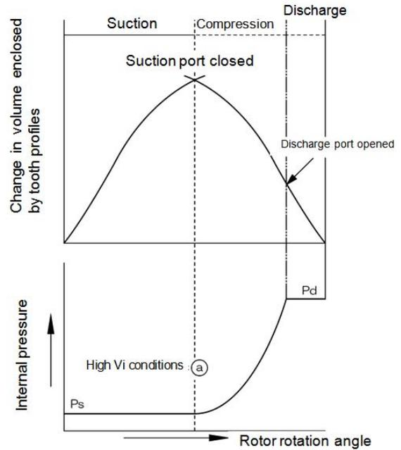
**(B) Improperly adapted  $V_i$  to load condition**
