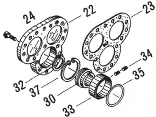
Figure 5-12 Balance Piston Block
