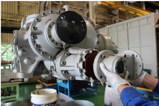
Photo 008 Removing Unloader
