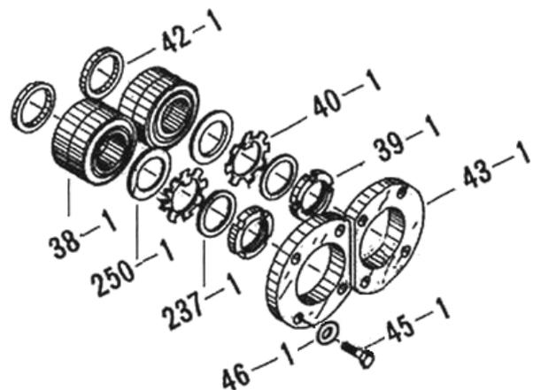
Figure 5-15 Low-stage Thrust Bearing Block
