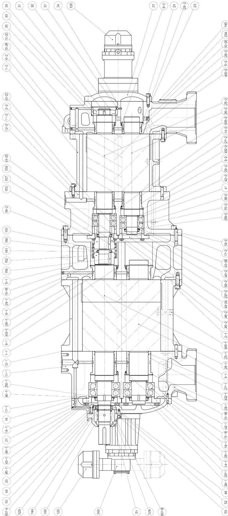
Figure 7-4 2520LLC Assembly Sectional View (Horizontal)
