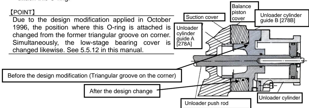
**Figure 5-21 Modification of O-ring Attaching Position**
