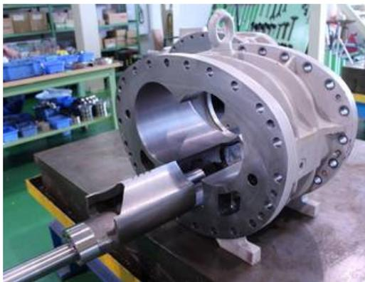
Photo 062 Installing Slide Valve (Low-stage)
