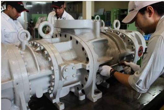
Photo 030 Tapping Alignment Pin
