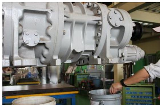
Photo 004 Draining Oil from Bearing Head
