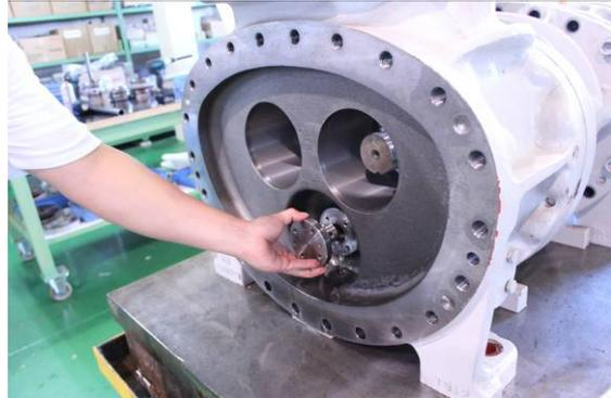
Photo 035 Removing Oil Injection Pipe Gland
