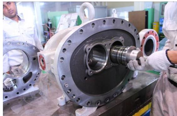
Photo 059 Removing Main Bearing
