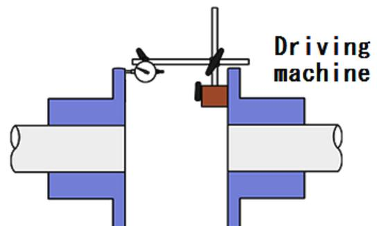
**Figure 3-4 Measurement of Angularity**
