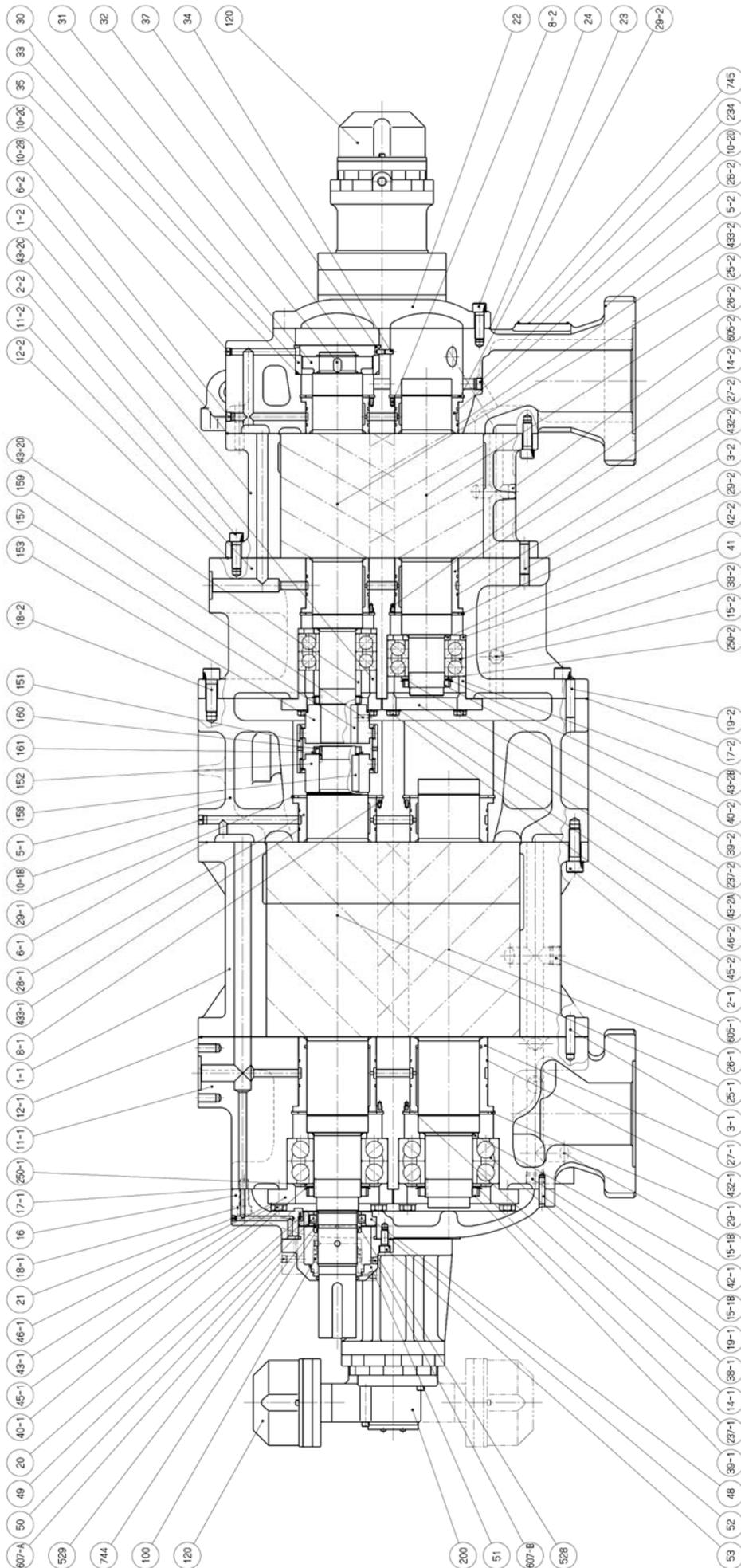
Figure 7-12 2520MSC Assembly Sectional View (Horizontal)
