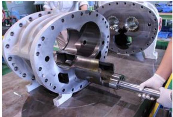
Photo 061 Removing Slide Valve Assembly
