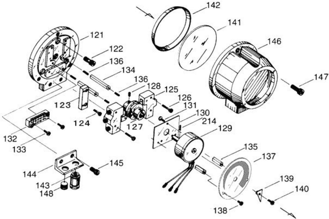
**Figure 5-3 Standard-type Unloader Indicator (High-stage Dial Plate)**
