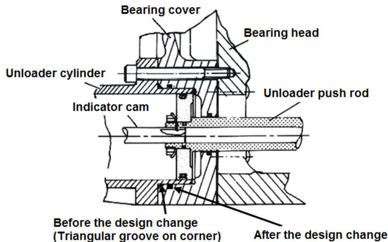
**Figure 5-23 Modification of O-ring Attach Position (Low-stage Unloader Cylinder)
