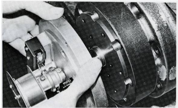
Photo 007 Removing Indicator Assembly
