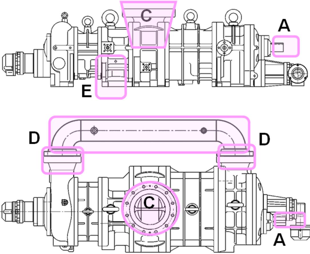
Figure 1-1 Locations of Hazardous Sources (Compressor)
