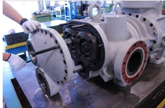
Photo 027 Removing Bearing Cover
