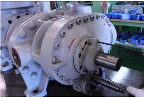
Photo 021 Separating Seal Cover with Eye Bolt
