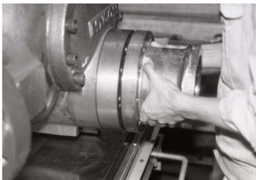
Photo 017 Removing High-stage Unloader Cylinder
