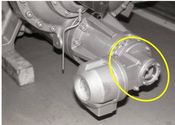
Photo 005 Low-stage Unloader Indicator Fixture (Circled Portion)
