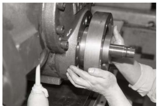
Photo 018 Removing Cylinder Guide B
