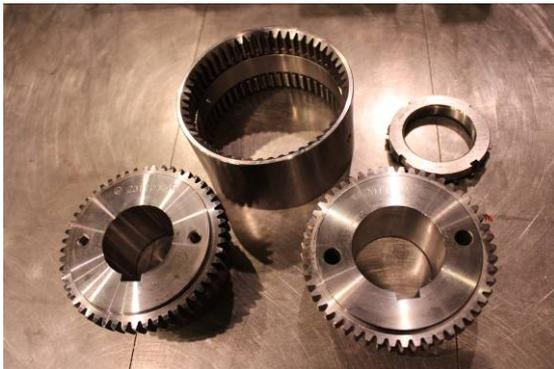
Photo 032 Current Gear Coupling Parts
