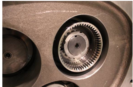
Photo 028: Low-stage Gear Coupling
