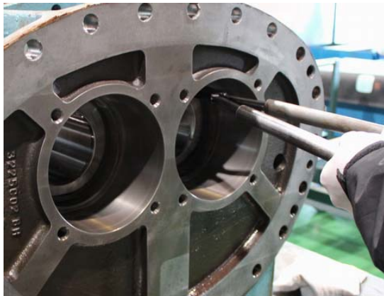
Photo 056 High-stage Bearing Head
