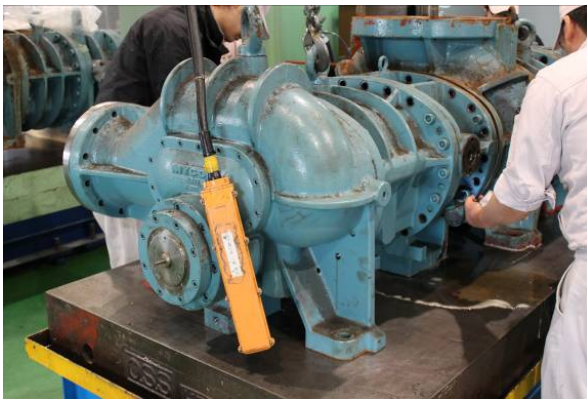
Photo 025: Screwing in the Bolts to Push and Separate
