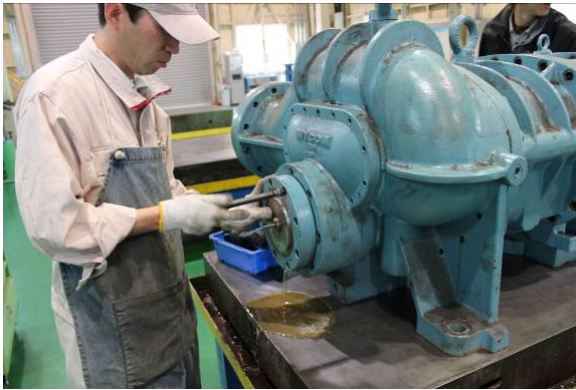
Photo 011: Removing the Unloader Cover
