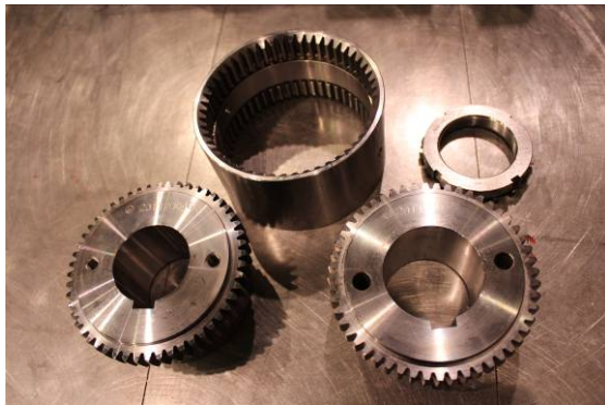
Photo 027: Current Gear coupling parts
