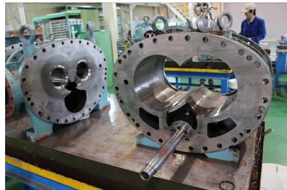
Photo 053 Removing the Slide Valve Assembly
