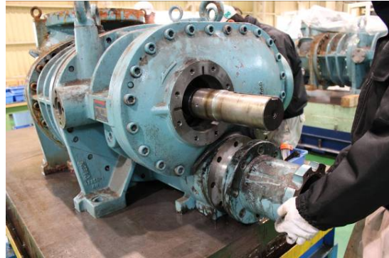
Photo 017: Removing the Low-stage Unloader Cylinder
