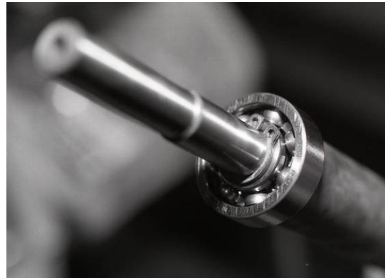
Photo 012: Ball Bearing for the Indicator Cam
