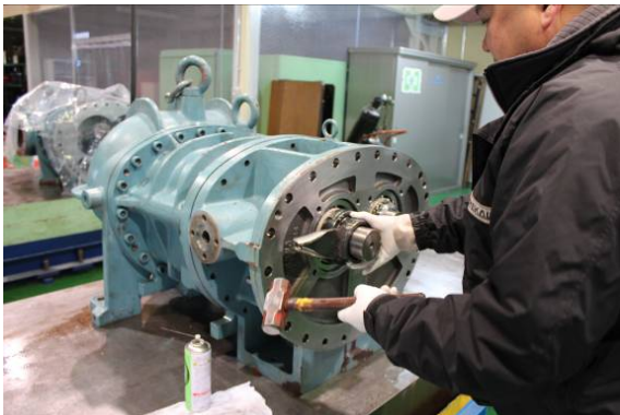
Photo 079 Tightening the High-stage Lock Nut
