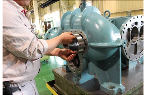
Photo 067 Installing the Balance Piston Sleeve
