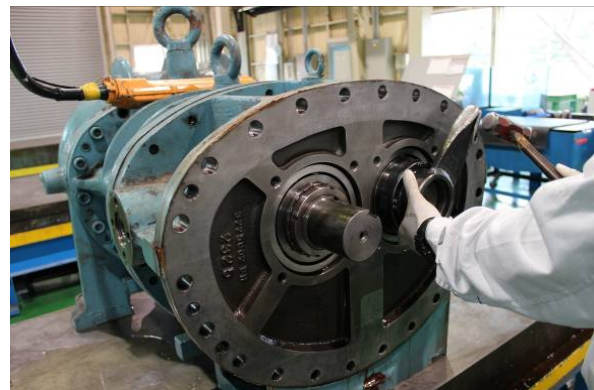
Photo 034 Loosening the Lock Nut
