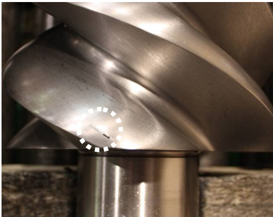
Photo 059 Mating Mark on the M Rotor
