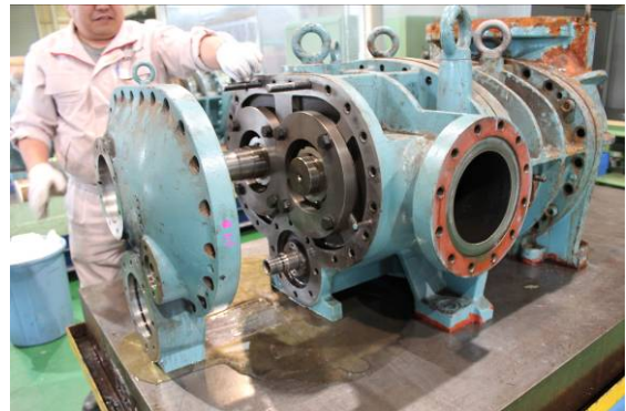
Photo 024: Removing the Bearing Cover
