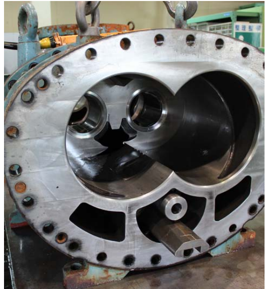
Photo 058 Low-stage Rotor Casing and Bearing Head
