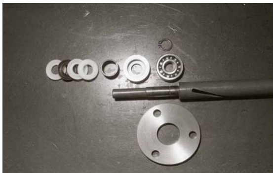
Photo 013: Indicator Cam Mounting Parts
