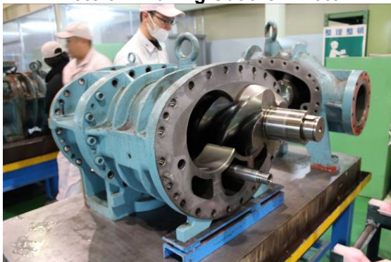
Photo 044 Pulling Out the M Rotor
