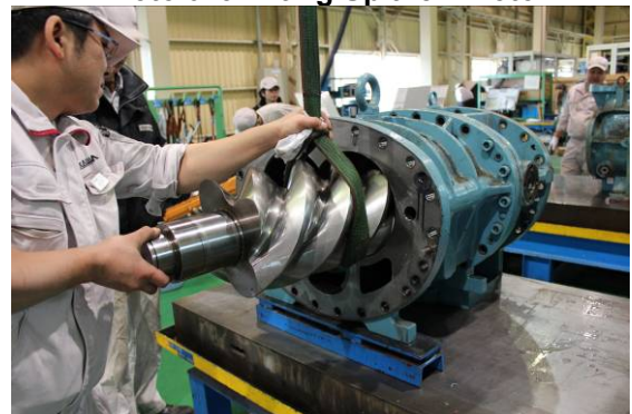
Photo 045 Lifting Up the M Rotor
