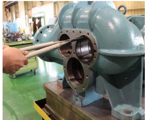
Photo 063 Installing the High-stage Snap Ring
