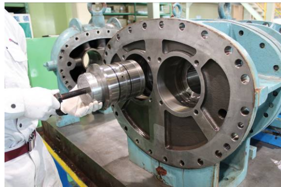
Photo 051 Removing the Main Bearing
