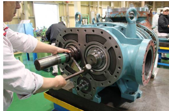
Photo 080 Tightening the Low-stage Lock Nut
