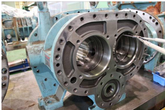
Photo 052 Removing the Snap Ring Internal
