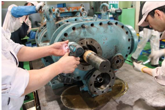
Photo 023: Removing the Bearing Cover
