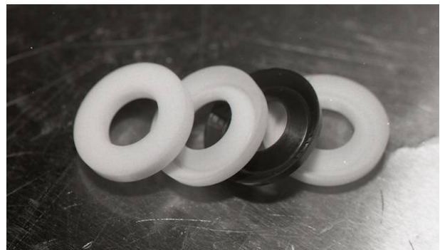
Photo 014: V-ring (Black part is NBR/FKM)
