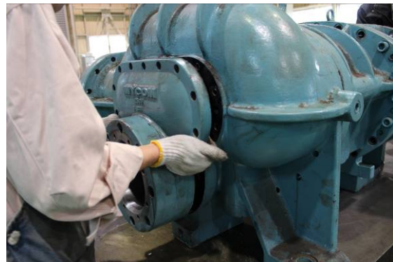
Photo 018: Removing the Balance Piston Cover and Unloader Cylinder together
