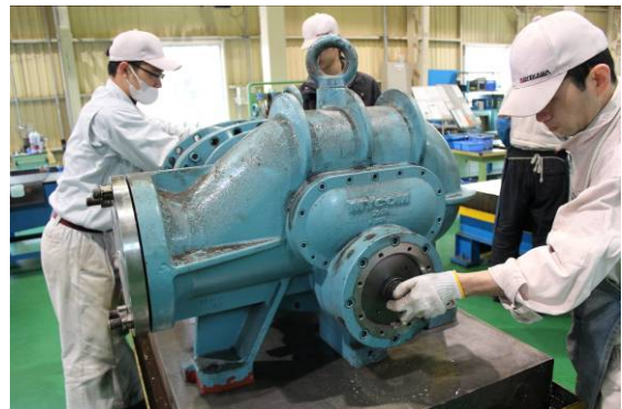
Photo 016: Use Lock Nut Wrench to Loosen the Lock Nut (High-stage)
