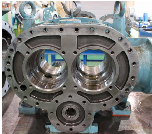
Photo 057 Low-stage Bearing Head
