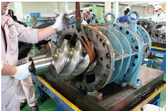
Photo 047 Pulling Out the Low-stage M Rotor
