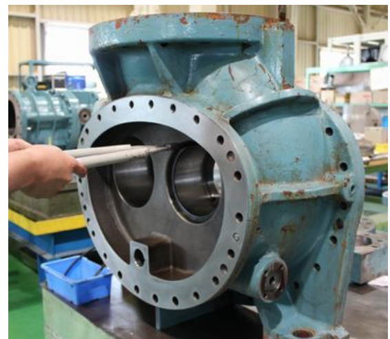
Photo 065 Installing the Low-stage Snap Ring
