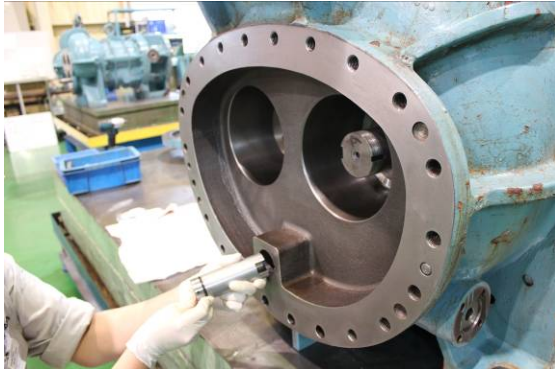
Photo 029 Removing Oil Injection Pipe
