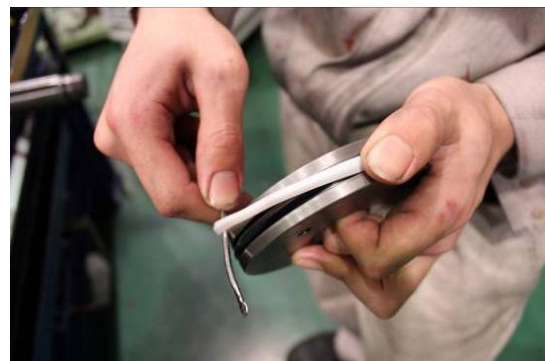
Photo 019: Removing the Cap Seal
