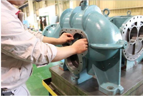
Photo 066 Installing the O-ring
