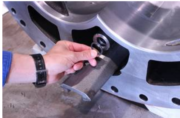
Photo 055 O-ring for the Oil Injection Pipe Guide
