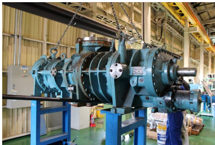
Photo 003: Loosening Lower Flange Fastening Bolts
