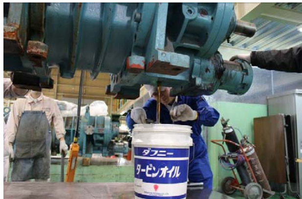
Photo 004: Draining Oil from the Bearing Head
