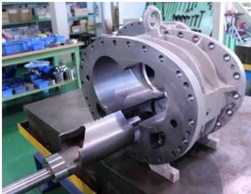
Photo 054 Installing the Slide Valve (low-stage)
