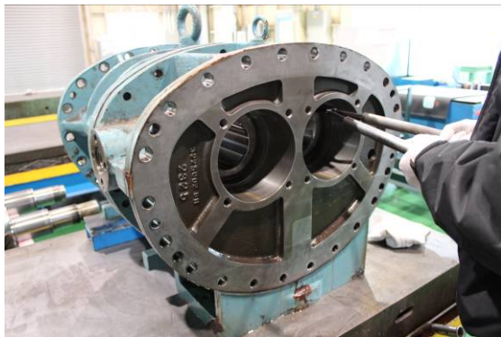
Photo 050 Removing the Snap Ring Internal
