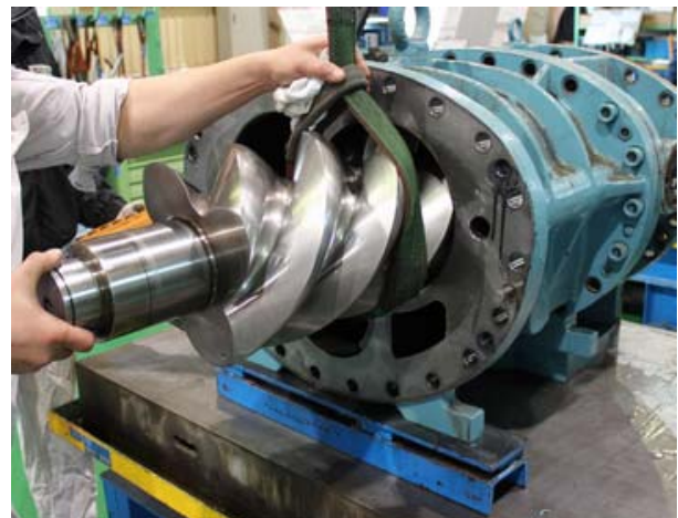
Photo 061 Installing the M Rotor
