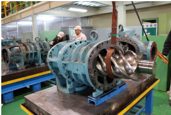
Photo 042 Pulling Out the F Rotor
