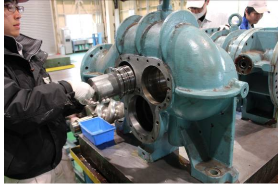
Photo 034 Removing the Side Bearing
