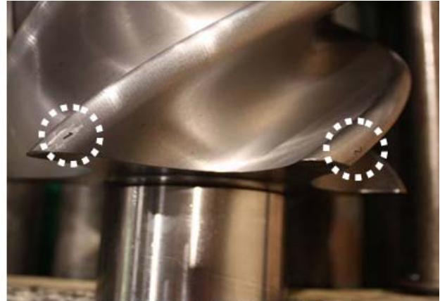
Mating Mark on the F Rotor
