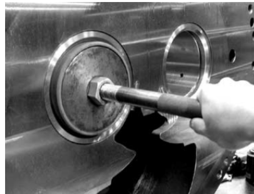
Figure 5-17 Example Tool for Press Fitting the Bearing
