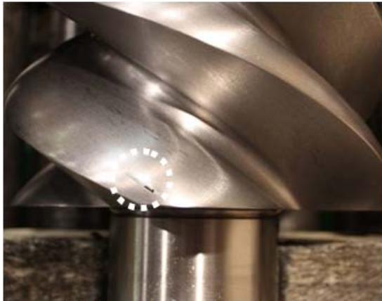
Mating Mark on the M Rotor
